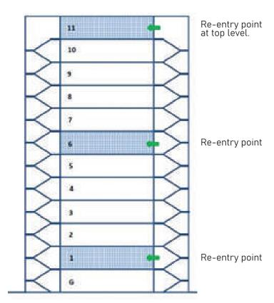
Figure 6.8.3.1 (a). Required re-entry floors when starting at the top level.
